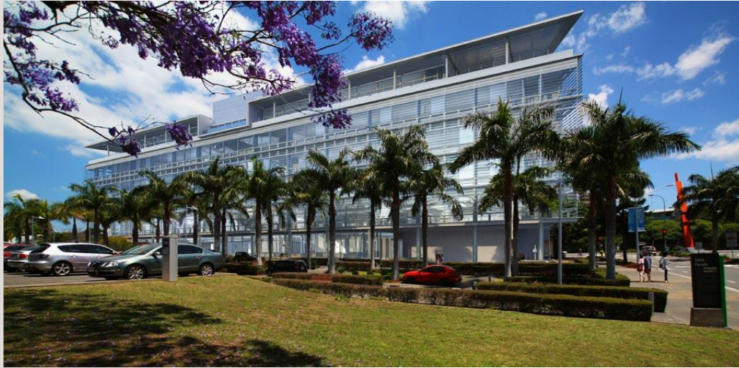
QUT CIP2, Kelvin Grove (rendering) Horizo motorised external venetian blinds mounted onto G.James custom curtain wall.
